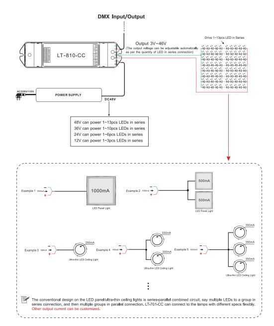
3) Connection Diagram for Multiple Decoders:
